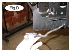
Remove three torx screws in each fender well (Fig. B). Disconnect the fog lights, if the vehicle is so equipped (Fig.D). Then, remove four bolts, two on the top of each frame tube (Fig.C). Now, remove two bolts on the bumper side braces on each side. These are located on the sides of the frame tubes.
