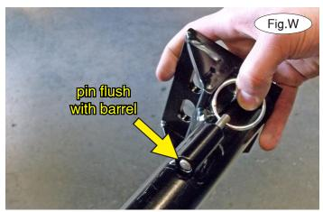
The spring-loaded pin on the removable arm snaps into a notch on the receiver, locking the removable arm into its final towing position. Before inserting each arm into the receiver, verify that the spring is working by ensuring that the spring-loaded pin moves easily back and forth within the barrel when pulled and that it can be pulled flush with the face of the barrel (Fig.V and Fig.W).
