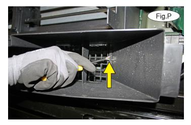
11. On each side, remove two 15mm (head) bolts attaching the bumper core to the frame (Fig.Q). Then, remove the foam covering and two 18mm (head) bolts and nuts attaching the tow hook to the frame. Note: the tow hooks will not be replaced. Retain the tow hooks and their hardware for replacement in case the bracket is ever removed.
