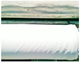
Align Awning Guard with the seam of the awning fabric and where it attaches to the RV. Have a helper hold the Awning Guard up along the seam (this will keep it straight).
