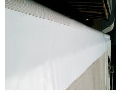
Lay cut ,Awning Guard along roof of RV.
