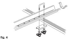
If your bike is not "centered" on the wheel tray then you should adjust by moving the bike support arm bracket along the wheel tray using the two fixing nuts/bolts. If you do this make sure the nuts are re-tightened firmly.
