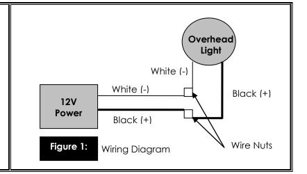
2. Connect the black wire to the positive wire and the white wire to the negative wire using wire nuts (Figure 1).
