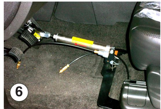
*Note:* some 2008 models with adjustable pedals may not require the adjusting arm on the air cylinder (Fig.1). Instead, it will mount directly to the mounting post, as shown in Figure 6.
