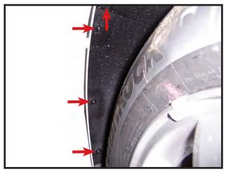
2. Remove four T20 Torx screws from each wheel well. (Driver's side shown)
