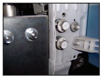
**15.** Reinstall bumper using the eight factory bolts that were removed in step 9.
