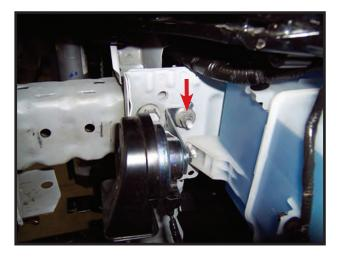
8. Remove nut from horn mount and let horn hang down.
