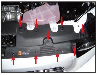
1. Remove six plastic push fasteners, four 10MM bolts, and eight phillips screws from top radiator cover. (Driver's side shown)
