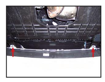
5. Remove two phillips screws from underside of facia now visible after removing front portion of belly pan.
