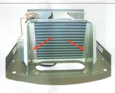
3. Remove (2) screws that hold evaporator to bulkhead.
