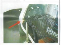
7. Secure heater lead with wire holder, as shown.
