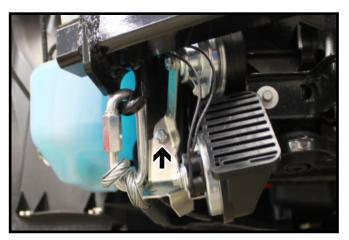
17. On the passenger side, reinstall the horn assembly to the vehicle. Use one of the existing holes on the frame below the baseplate with a 1/4"-20 x 3/4" bolt and 1/4" nylon nut.
