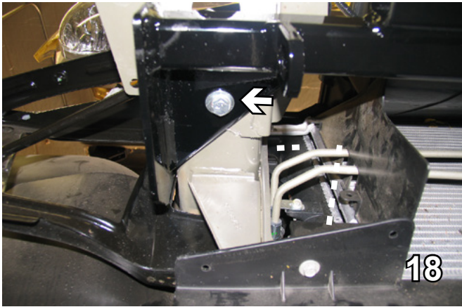
18. Insert 3/8" nut plate into frame end to align with drilled hole and tighten 3/8"-16 x 1 1/2" hex bolt, 3/8" flat and lock washer.
