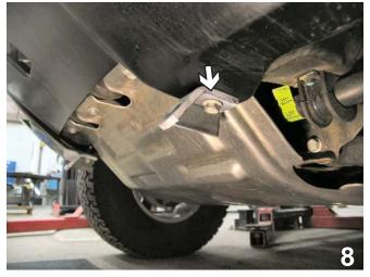
8. Reinstall the metal bumper fascia using upper existing bolts but do not tighten completely. Install the convenience link weldment to the lower existing bolt, tighten all bolts completely and reinstall the rubber inserts, fog lights and grill insert.
