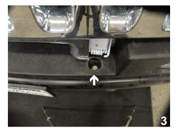
3. Using the 18MM socket, remove one metric bolt from the top of the bumper. Do this to both sides of the vehicle. Set bolts aside to be reinstalled later.
