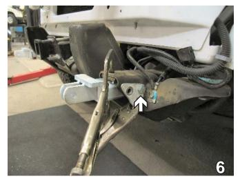
Insert the baseplate weldment into the tow hook opening and align the backing plate with the outside tow hook hole, 1/4" forward of the frame rail, clamp in place and install the 4 1/2" hex bolt, 1/2" lock washer and 1/2-13 hex nut. Do this to both sides of the vehicle.
