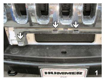
Pull the center grille insert forward to release the four clips, one on each side and two in the middle. Set insert aside to be reinstalled later. The passenger's side is shown in the photo above.
