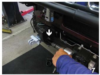
7. Using the baseplate weldment as a template, drill through the forward existing hole on the inside of the frame rail with the right angle drill and the 17/32" drill bit. Do this to both sides of the vehicle. If a right angle drill is not available, it may be necessary to remove the winch bracket to allow room for drilling.
