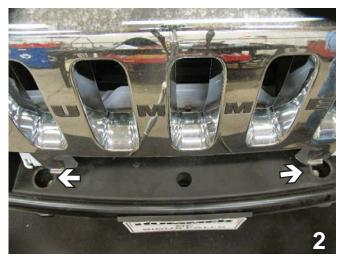
2. Remove the two rubber inserts from the top of the bumper. Set the rubber inserts aside to be reinstalled later.
