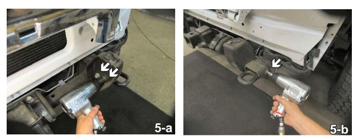
5. Using the 18MM socket, remove three metric bolts from the tow hook, two on the inside (see photo 5-a) and one on the outside (see photo 5-b). Pull tow hook forward and set aside. Do this to both sides of the vehicle. The tow hooks will not be reinstalled. Please return them to the customer.
