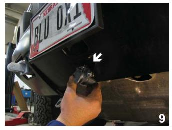
9. Using the 1" self tapping screw, install the electrical bracket just below the license plate bracket while ensuring enough clearance for the bracket cover to open.
