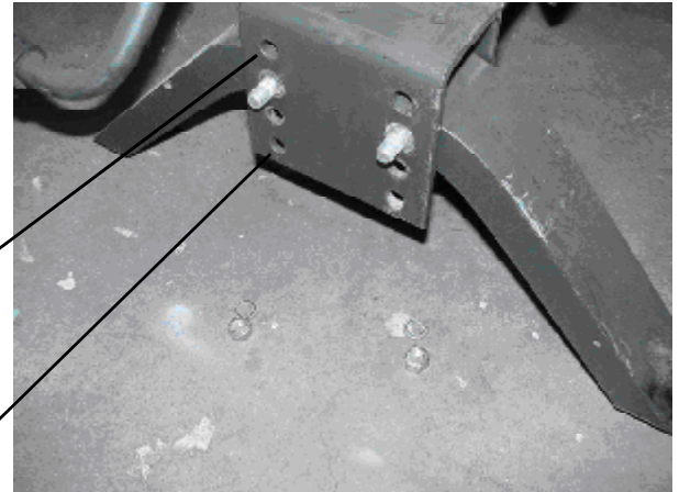
Figure 2-Left Side Frame Mounting Nuts removed
