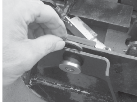
Figure 23 – Installing Front Nylon Spacer
