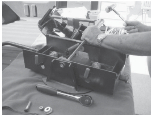
Figure 13 – Removing Thick Bushing
