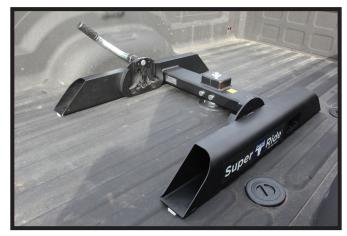
2. Place the base of the hitch onto the gooseneck 2-5/16" hitch ball.
