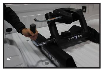
Release locking handle by pulling the handle towards the rear of the truck bed. Then pull the handle outwards and then towards the rear of the truck bed again.
