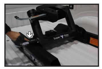
2. The handle is now locked into the grove on the side of the tubing.
