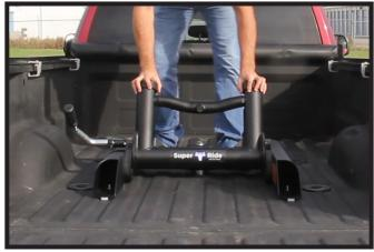
Move the shock towers towards the cab of the truck and manually reengage the the locking handle.
