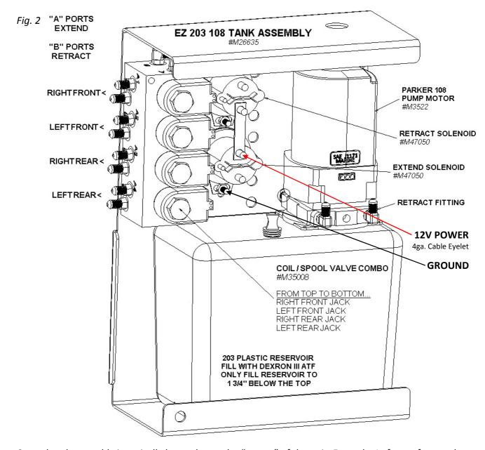
Central tank assembly is typically located near the "center" of the unit, Example: In front of rear axle on driver's side frame rail (outside of rail or between rails).
