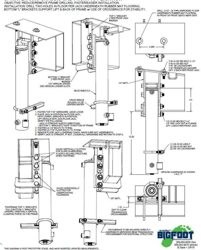
System: Rear Jack Setup for Channel Series Cylinders (N/A for all applications)
