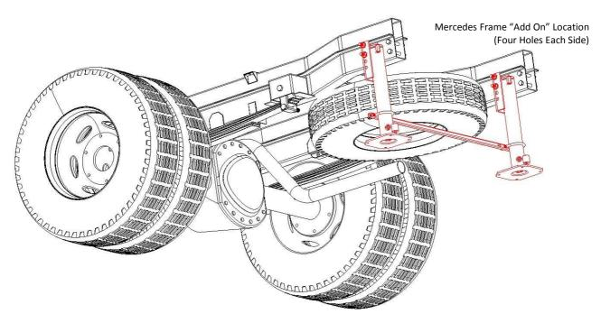
Remove old hardware (two bolts per side), Mount jacks utilizing existing holes by utilizing included longer hardware (1/2" Grade-8 6 ½" Bolts & Flange Lock Nuts). Crossbrace is required.
