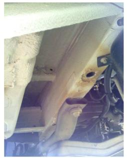
Passenger side jack location (under cab) cylinder also mounted on the outside face of the frame. Removal of the storage box in the step rail (shown in picture) must be removed. Angle drill will be required for 5/8" or 3/4" hardware.
