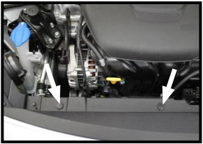
1. Remove the five (5) push pins that are located in the front area, underneath the hood. There are three (3) push pins located on the outer edge of the driver side and two (2) on the outer edge of the passenger side.
