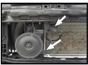
6. Unplug the horn and temperature sensor. They will be repositioned after the baseplate has been completely installed.
