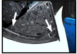
4. Remove the two (2) push pins located under the bumper towards the outer edge. Do this on both sides.
