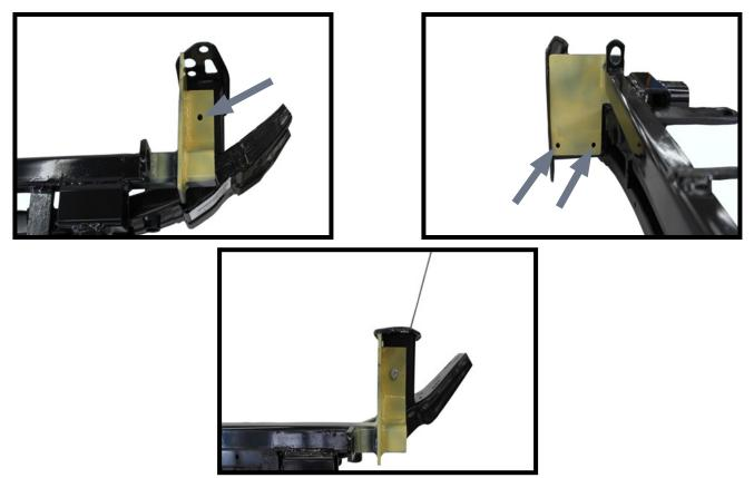
11. Place baseplate onto bumper frame. The back edge of the baseplate should be flush with the bumper frame bracket. Using a 13/32" drill bit and the baseplate as a template, drill out the holes. Do this on both sides.
