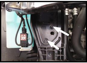
7. To remove the front bumper, unclip the wiring harness and place it out of the way. Next, remove the bumper using a 12MM socket for the two (2) outer bolts and 10MM socket for the center bolt on the top of the bumper frame bracket. On the bottom of the bracket there are two (2) 12MM bolts that need to be removed. Do this on both sides of the vehicle.
