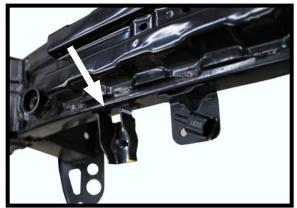
10. Remove the horn bracket located on the passenger side. The horn will be relocated after the baseplate has been installed.
