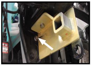
12. Reattach the bumper frame using the existing hardware except for the top bolt on the bottom section of the bumper bracket. The supplied 8MM bolt replaces the bolt that was removed as the attached washer would not allow the bolt to be started.
