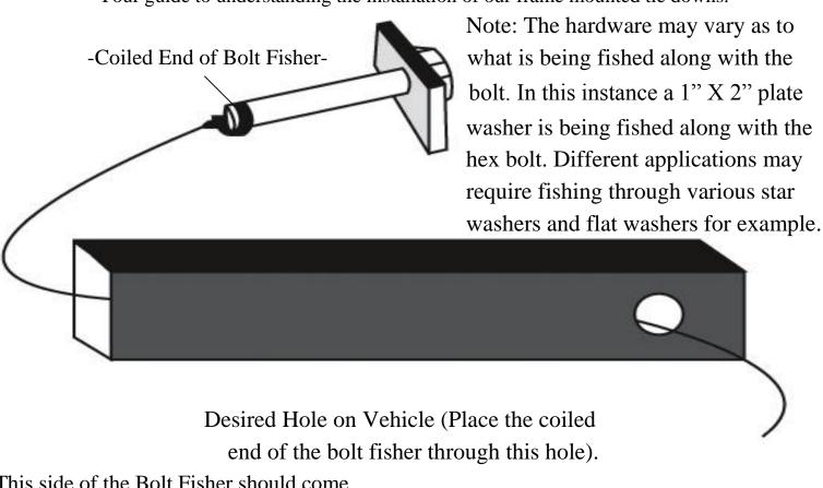
This side of the Bolt Fisher should come out of a hole where the required hardware (for example 1" X 2" plate washer) can pass
