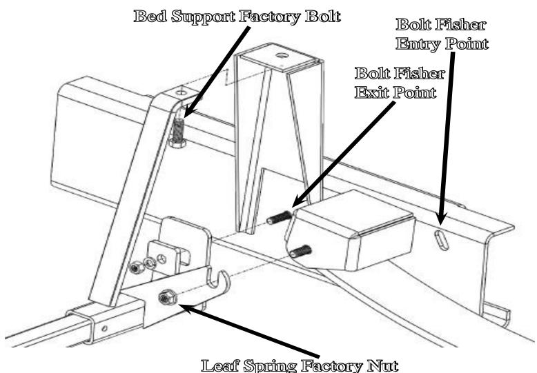
Leaf Spring Factory Nut (Don't remove, loosen 3/8")
