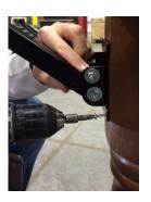
6. Using the provided screws secure the Chair Buddy™ to the post only screwing in the bottom two screws.
