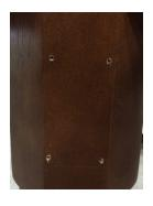
5. With a 7/64th drill bit drill a pilot hole approximately 1" deep for all four screw locations. (Must drill pilot holes or table post may split).
