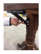
2. Position Chair Buddy™ against post where Chair Buddy™ is as high as possible on the post. T-handle should be touching the underside of table. (Zip tie must still be uncut). Mark with a pencil the bottom of the mounting face.
