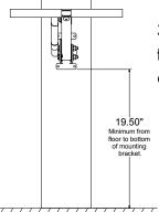
3. Measure from the line to the floor to ensure it is a minimum of 19.5".
