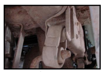
15. Reinstall the factory exhaust bracket. If the exhaust pipe sits too high and interferes with the hitch, cut the rubber hanger off of the exhaust bracket and install the supplied adjustable exhaust hanger Reinstall the spare tire per the vehicles owners manual.
