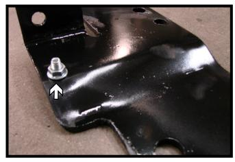
10. Install the 5/16" carriage bolt thru the square hole in the driver side plate with the nut on the outside.
