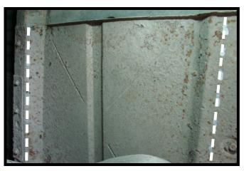
5. If equipped, trim and discard the exhaust heat shield in the area shown.
