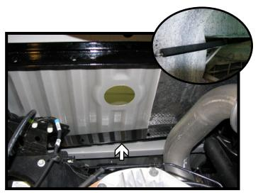
Slide each cross member in on top of the frame on the driver side just in front of the wheel well (inset).
