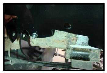
11. Slide the side plate in between the frame and the outer hook of the j-clamp, and position it into the studs of the crossmembers and the j-clamp. Do this on both sides of the vehicle.
