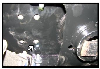
13. Using a 19/32" drill bit, drill the two (2) holes closest to the ball thru the bed. Do this on both sides.
