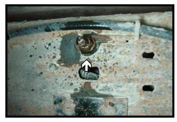
4. Using a 15MM socket, remove the nut from the emergency brake holder.
