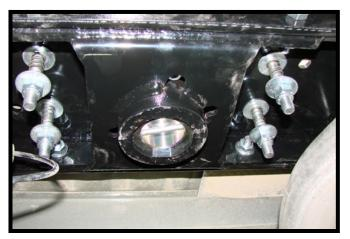
14. Insert the 1/2"-13 u-bolts thru the holes from the topside. Install a 1/2" flat washer, spring, another 1/2" flat washer and 1/2"-13 lock nut onto each u-bolt stud. Tighten until the washers are touching the spring without compressing it.
