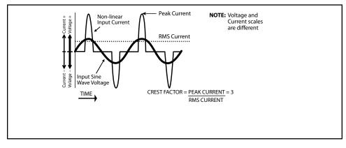
Fig 1.3 High Crest Factor of current drawn by SMPS
