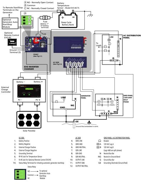
Fig 3.13 Typical Shore Based Installation
