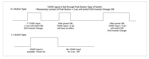
Fig 4.8. On/Off Logic Diagram for Remote Switch Options
