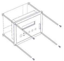
Flush mounting the EVO-RC on the wall with 4pcs,  $\Phi$ 3mm self-tapping screws (flat head).
