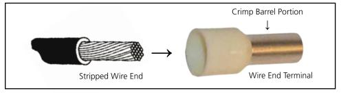
Fig 3.11 Stripped Wire End Terminal on AC Wiring
