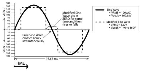
Fig 1.1 Pure and Modified Sine Waveforms for 120V, 60 Hz
