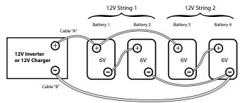
Fig. 3.7 Series-Parallel Connection
