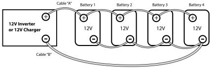
Fig 3.6 Parallel Connection
