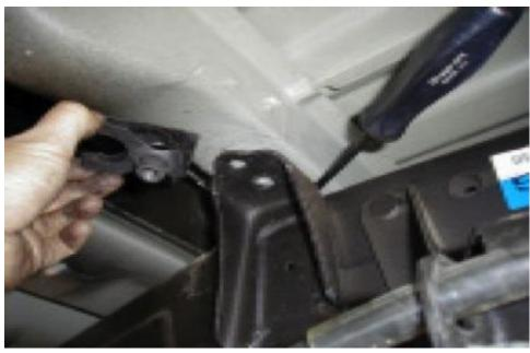
To remove nut plate, insert screwdriver as shown. Pry down on screwdriver and slide out nut plate. You will not reuse factory nut plate.
