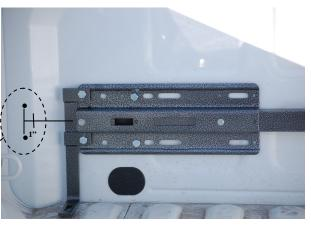
**STEP 8** – [*Hardware Kit D*] Drill 3/8" dia. Hole through frame brace foot , bed, and frame/bed cross member 3 inches
