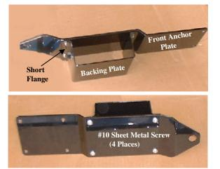
Remove board from between bed & cab and slide black front anchor plate assembly into place. Reset the frame braces on each end of the assembly. Start but do not tighten all 4 bolts through guide plate and frame braces. into threaded holes in black anchor plate.
