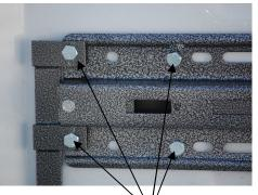
3/8" fine thread bolts through bed front wall into black anchor plate **STEP 7** – [*Hardware Kit J*] Using the #10 self drilling & self tapping screws, install 2 screws through bed front wall into the black anchor plate at the locations shown.
