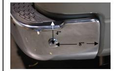
Flat edges of Anchor Bolt must be horizontal.
