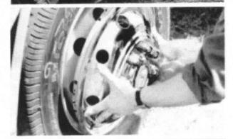
Set the FastLiner<sup>TM</sup> in position at the base of the wheel and tip it up onto the wheel making certain that the valve stem cut out is properly aligned with the valve stem.
