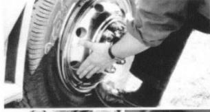
Holding the bottom of the FastLiner<sup>TM</sup> in position with one foot, use slight pressure with your hands to start the retention ring into the wheel. The retention clip will begin to engage the wheel.
