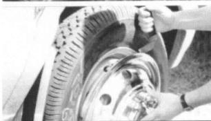
Move around FastLiner<sup>TM</sup>, prying at retention clip locations until FastLiner<sup>TM</sup> is loose. In order to prevent damage, do not allow FastLiner<sup>TM</sup> to fall to the ground upon removal.
