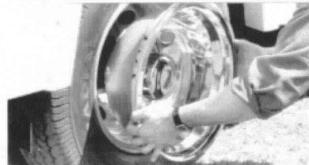
Align the openings in the rear FastLiner<sup>TM</sup> with the openings in the wheel.
