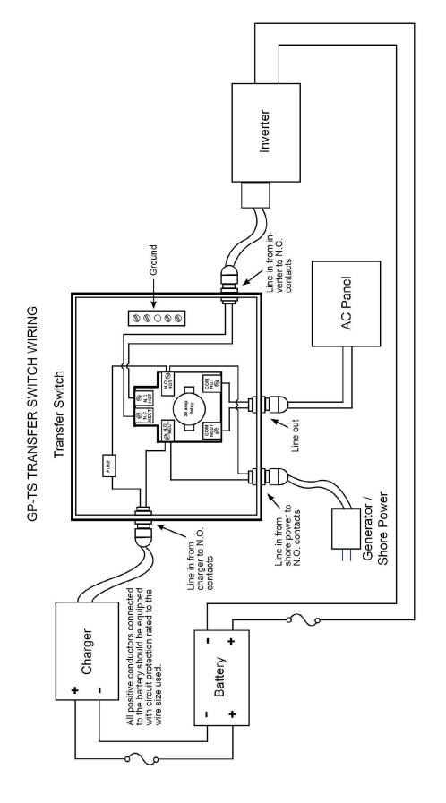
If the inverter supplies power to the AC panel which in turn provides power to a converter, the resulting battery loop will quickly drain the batteries. Disconnect the converter entirely from the system or rewire the converter to the N.O. contacts of the transfer switch. Make sure there is an AC fuse in line to protect the circuit.
