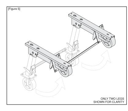
Swing Spring loaded Legs to nested position and release the Engagement Tab into the notch to secure [Figure 5 & 6].
