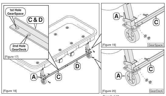
**GEARSPACE:** Install using the holes **closest** to the end of the Right & Left Support Bars [**C & D**] [Figure 17 & 19].
