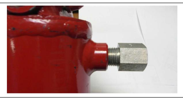
Picture of SAE fitting in a Jack-Notice that there are no threads exposed between the cylinder body and the hex on the fitting.
