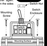
Next, mount the switch in the switch enclosure (or your own panel), securing it with one switch nut. Use the two mounting screws to attach the enclosure (if used) to a flat mounting surface, after routing all wires out the small slot on the side.
