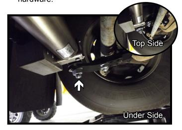
5. Install the solenoid end of the TruCenter to the end bracket with a 3/4"-10 x 3-1/2" bolt, 3/4" washers and 3/4" lock nut provided with the TruCenter. Install the other end of the TruCenter onto the tie rod bracket with a 3/4"-10 x 3-1/2" bolt, 3/4" washers and 3/4"-10 lock nut provided with the TruCenter.
