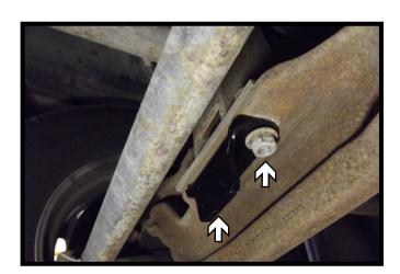
Remove the two (2) existing nuts from the axle. Install the base bracket onto the axle and reinstall the existing nuts. Tighten to manufacturer's specifications.
