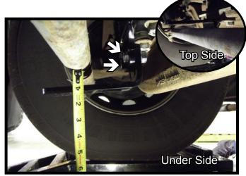
3. Install the center bracket to the base bracket with the 1/2" hardware onto the top side or under side of the tie rod depending which gives the TruCenter better clearances on your particular motorhome model. Insure there is a minimum 1" gap between the center bracket and tie rod. Fully tighten the hardware.
