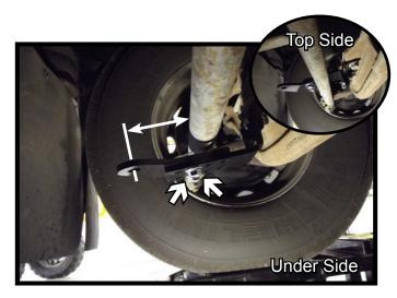
Attach the tie rod bracket to the tie rod with the u-bolts and nuts from the appropriate u-bolt kit. DO NOT tighten. Measure the distance from the tie rod to the installation hole. (not shown)
