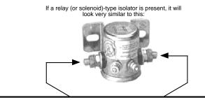
At the factory, the manufacturer has connected one of these large terminals to the Positive terminal of your house battery battery(s). You want to connect Trik-L-Start's YELLOW wire to the terminal that goes to the HOUSE batteryies, and connect Trik-L-Start's BLUE wire to the terminal that goes to the STARTING battery(s).
